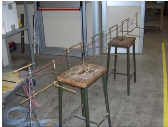
Figure 1: Positioning of the strain gauges over the metal support.
