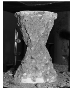
Figure 2. Concrete specimen at the end of the test, after removal of the outer part.
