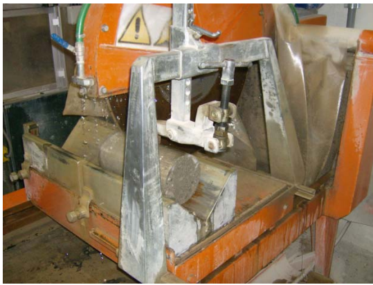
Figure 32: Automatic cylinder-end grinder
