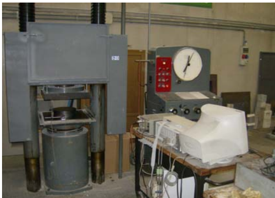
Figure 36: Compression-testing machine and acquisition apparatus
