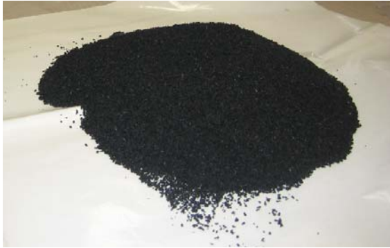
Figure 28: Gommamica®Powerfill ECO (SBR Styrene Butadiene Rubber) rubber coarse aggregate, commercialized by Elastrate Srl
