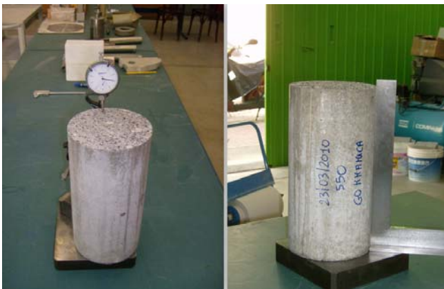
Figure 33: Analogical centesimal comparator and carpenter's square for checking planeness and perpendicularity
