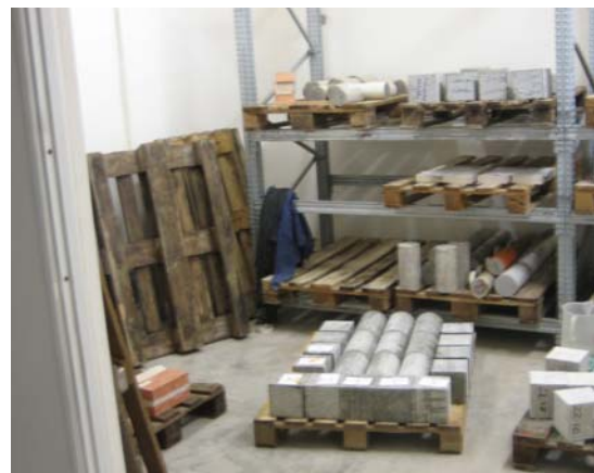
Figure 31: Curing room under controlled thermohygrometric conditions
