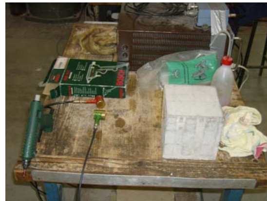
Figure 34: Hot glue gun loaded with a glue stick and probes for microseismic analysis: the red probe is the transmitting sensor, while the green probe is the receiving sensor
