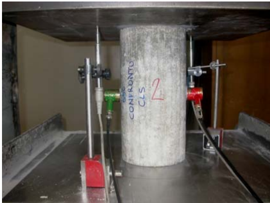
Figure 35: Positioning of the instrumented cylindrical specimen on the compression-testing machine
